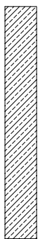
PROFILE 330-T 8 LBS. PER LINEAR FOOT ONE SIDE COULD BE SPLIT IN LIEU OF SMOOTH
