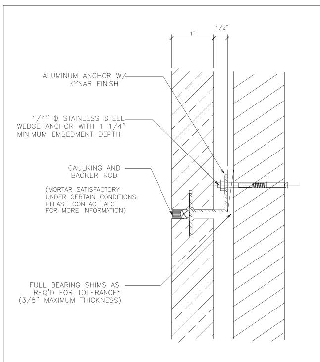
1 INTERMEDIATE STONE ANCHOR FOR USE @ C.M.U. BLOCK BACK-UP
