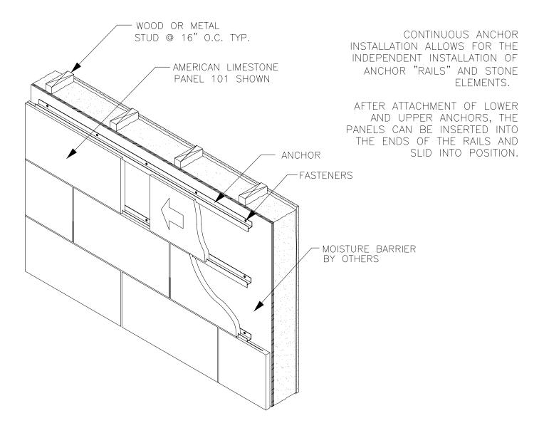
FASTENER HOLES SHOULD BE DRILLED NO MORE TAN 16" OC AND CENTERED IN THE "V" GROOVE PROVIDED. FASTENER TYPE AND REQUIREMENTS SHOULD BE CONFIRMED USING THE ANCHOR LOADING TABLES IN THE ALC SOLUTION MANUAL (SEE P.3.1.3 AND 3.1.3A) OR PER AN ENGINEER'S RECOMMENDATIONS.
