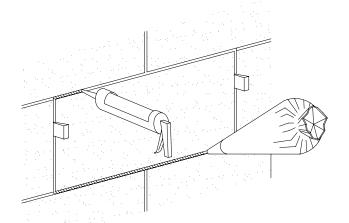
USE TEMPORARY SHIMS OR WEDGES IN THE VERTICAL JOINTS TO POSITION THE PANEL.
